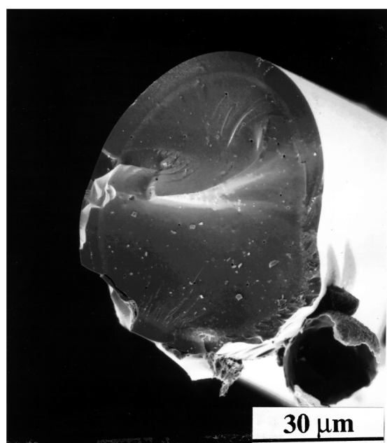
Fig. 11 SEM micrograph of a TVS-PMS fiber (10 wt.% of TVS added) heated to 1000^\circ\text{C} for 1 h in Ar.
